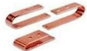
Silver, tin or nickel plating for Tinned Copper Bus Bars is necessary in high temperature applications. At DC to 60Hz there is some controversy as to which plating is the best because while silver has the highest conductivity, it is also more noble than copper so it will actually accelerate corrosion wherever the plating gets scratched. Thus, you don't want to just use toothed lock washers, for example, in between a nut and the bus bar (i.e. - use a flat washer, too).
